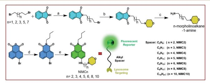
Scheme 1 Schematic representation of the synthesis of NIMCs, and the corresponding general conditions are as follows: (a)  $K_2CO_3$ , dry MeCN, reflux, 8 h, 78–83%; (b) morpholine,  $K_2CO_3$ , dry DMF, 100 °C, overnight, 84–91%; (c)  $N_2H_4\cdot H_2O$ , EtOH, reflux, 2 h, quantitative yield; (d) n-butylamine, EtOH, reflux, 2 h, 77%; (e) N-morpholinoalkane-1-amine, dry DMSO, 105 °C, overnight, 51–57%.
