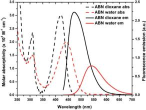
Fig. 4 Absorption (dashed line) and emission (solid line) spectra of ABN in dioxane (black) and water (red). The integral areas of emission spectra are normalized to brightness  $\epsilon \cdot \Phi_{em}$ .
