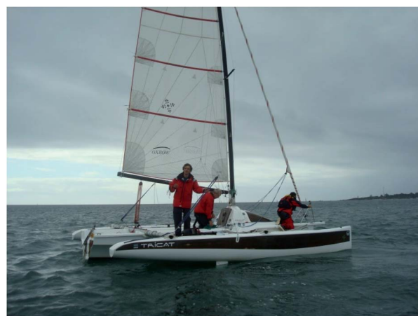
Fig. 3 Gwalaz, flax fibre reinforced trimaran.
