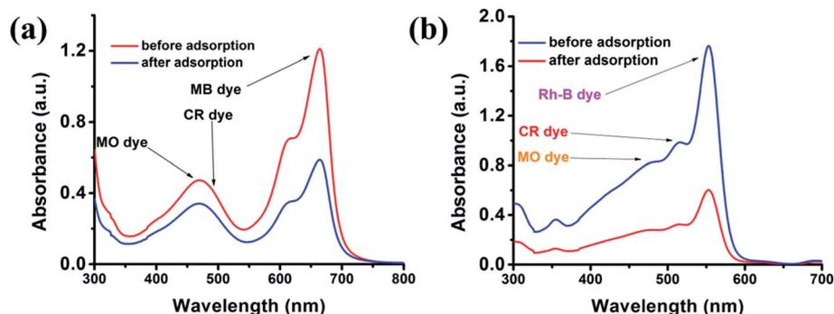
Fig. 9 Adsorption plots of MB (a) and Rh-B (b) in the presence of CR and MO dyes.
