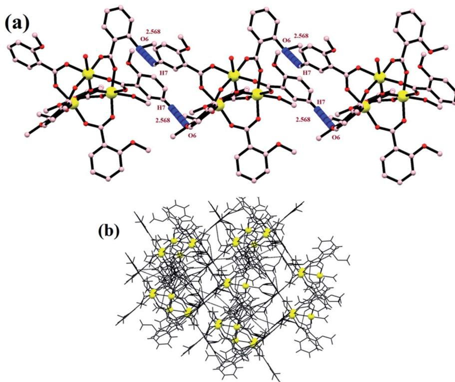
Fig. 4 (a) A 1-D zig-zag chain and (b) a supramolecular network formed by non-covalent interactions.
