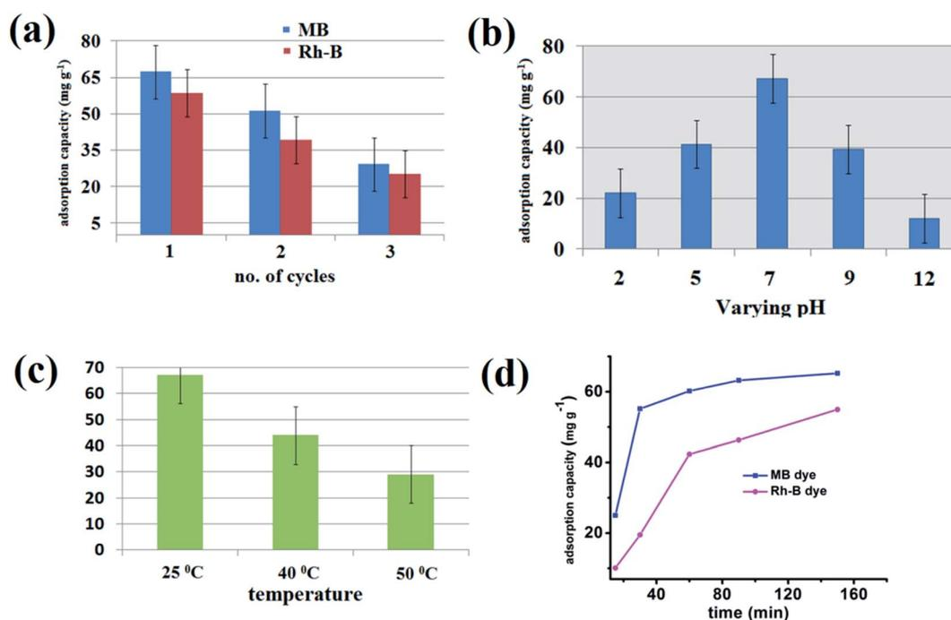
Fig. 10 Recyclability graph of the adsorbent (a), graph for the effect of pH (b), graph for the effect of temperature (c) and the plot showing effect of contact time (d) on the adsorption process.
