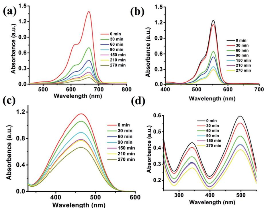
Fig. 7 Adsorption titration plots of organic dyes *i.e.*, MB (a), Rh-B (b), MO (c) and CR (d) recorded on a UV-visible spectrophotometer using the  $\{\text{Fe}_3\}$  cluster as the adsorbent.
