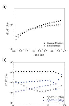
Fig. 2 (a) Rheology time sweep (10% strain, frequency of 1 Hz) at 25 °C to characterise gelation time of  $C_6E-3T-1:1$  using 1 mol% DBU. (b) Frequency sweep analysis showing storage and loss modulus *versus* frequency for networks synthesized using DBU or NEt<sub>3</sub> at 25 °C (1% strain from 0.1 to 10 Hz, or 0.06 to 62 rad s<sup>-1</sup>).
