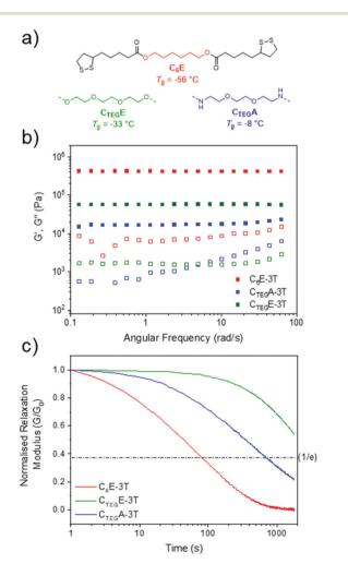
Fig. 4 (a) Structures of monomers to make networks at 8:1 ratio. (b) Rheology frequency sweep of networks at 25 °C (1% strain from 0.1 to 10 Hz, or 0.06 to 62 rad s<sup>-1</sup>). (c) Stress relaxation experiments at 2% strain. 100 °C.
