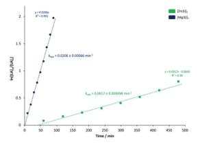
Fig. 3 Pseudo-first-order logarithmic plot for the polymerisation of rac-LA at 80 °C in toluene {[rac-LA]: [M]: [BnOH] = 100:1:1} using [Zn(1)]<sub>2</sub> and [Mg(1)]<sub>2</sub>. N.B. [LA]<sub>0</sub> = 0.69 mol dm<sup>-3</sup>.
