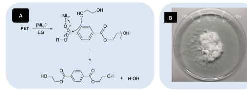
Fig. 7 (A) Metal mediated glycolysis of poly(ethylene terephthalate) (PET) into bis(2-hydroxyethyl) terephthalate (BHET) in the presence of ethylene glycol (EG), where R denotes the growth polymer chain. (B) Example of recycled product (BHET).
