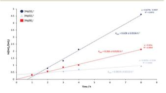
Fig. 6 Pseudo-first-order logarithmic plot for the degradation of PLLA cup using  $[Mg(1)]_2$  and  $[Mg(3)]_2$  in THF at 80 °C.  ${}^a[Mg(1)]_2 = 4$  wt% cat. loading (0.29 mol% relative to ester linkages).  ${}^b[Mg(1)]_2 = 8$  wt% cat. loading (0.57 mol% relative to ester linkages).  ${}^c[Mg(3)]_2 = 8$  wt% cat. loading (0.53 mol% relative to ester linkages).
