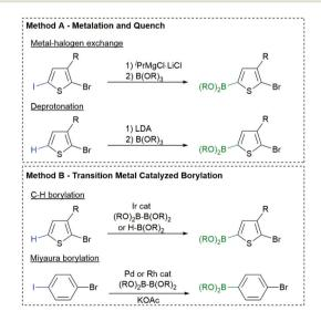
Fig. 2 Common methods used to synthesize halogenated aryl boronic esters. Abbreviations: 'PrMgCl = isopropylmagnesium chloride and KOAc = potassium acetate. Generic borate esters are represented as B(OR)<sub>3</sub> and diboron reagents as (RO)<sub>2</sub>B-B(OR)<sub>2</sub>.
