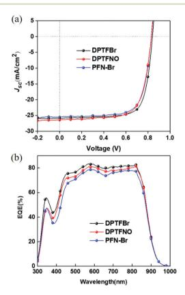
Fig. 6 J-V and EQE curves of devices with DPTFBr, DPTFNO, and PFN-Br as the cathode interlayer.
