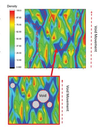
Fig. 5 Water/formaldehyde bubble migration due to material density formation.
