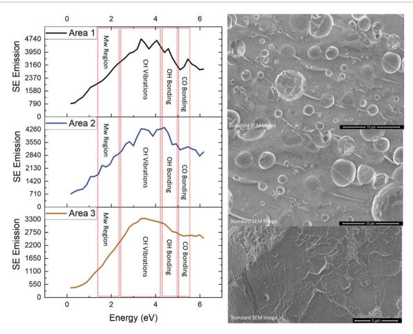
Fig. 1 Secondary electron spectra with accompanying SEM images for PR382 area 1, 2 and 3 highlighting SE regions identified as associated with functional group emissions. Area 1 & 2 HFW = 30  $\mu$ m whereas area 3 HFW = 25  $\mu$ m.
