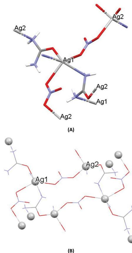
Fig. 3 (A) Molecular diagram of AGU. Selected bond lengths (Å) and angles [°]: Ag1–O1 = 2.492(7), Ag1–O2 = 2.845(6), Ag1–O4 = 2.425(5), Ag1–O8 = 2.340(5), Ag1–N4 = 2.636(8), Ag1–N3\_d = 2.657(8), O1–Ag1–O2 = 47.44(16), O1–Ag1–O4 = 130.89(19), O1–Ag1–O8 = 97.40(19), O1–Ag1–N4 = 91.6(2), O1–Ag1–N3\_d = 81.2(2). (B) Covalent Ag–O and Ag–N intra-molecular interactions lead to supramolecular assembly.
