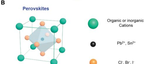
Fig. 2 Schematic illustration of solution-processable optoelectronic materials. (A) Structural representation of conjugated polymer (P3HT) with different molecular orientations (*i.e.*, edge-on, face-on and chain-on orientation) for different directions of charge transport and their corresponding optoelectronic applications. (B) Structural representation of perovskite, ABX<sub>3</sub> where A is methylammonium (MA), formamidinium (FA) or Cs, B is Pb or Sn, and X is Cl, Br or I.
