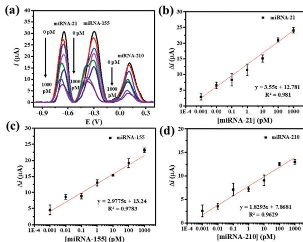
**Fig. 5** (a) SWV responses of the proposed biosensor after incubation with different concentrations of miRNA-21, miRNA-155, and miRNA-210, and (b), (c) and (d) corresponding calibration curves of the triplet assay towards miRNA-21, miRNA-155, and miRNA-210 respectively, in 10 mM PBS solution (pH 7.4).
