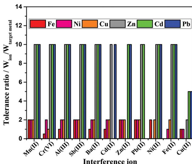
**Fig. 6** Tolerance ratio of heavy metal detection considering the interference ion  $\leq 10\%$ , using target metals solutions of  $500 \mu\text{g L}^{-1}$  for Zn(II), Cd(II), Pb(II) and  $5.0 \text{ mg L}^{-1}$  for Fe(II), Ni(II), Cu(II).
