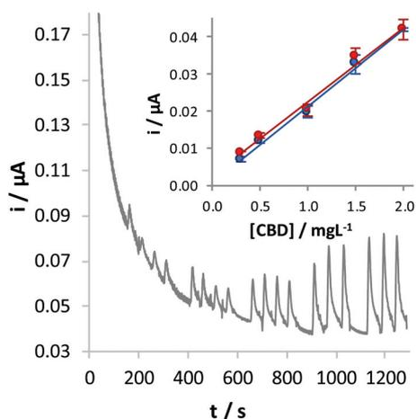
**Fig. 5** Amperometric response obtained in FIA by polarizing the GC/CB electrode at +0.70 V and injecting CBD solutions in the 0.3–2  $\text{mg L}^{-1}$  concentration range. The inset reports relevant calibration plots obtained by analysis of solutions at increasing CBD concentration (blue) or randomizing these analyses (red).
