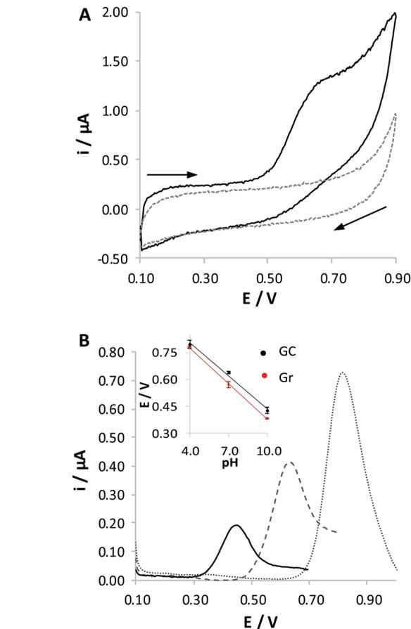
**Fig. 1** (A) CV response recorded in the presence (solid line) and in the absence (dashed line) of 0.1 mM RC, 0.1 M BRB (pH 7.0) at the Gr electrode, 0.050 V s<sup>-1</sup> potential scan rate. (B) DPV responses recorded in similar solutions at the GC electrode, at different pH values: 4.0 (dotted line), 7.0 (dashed line) and 10.0 (solid line), 0.015 V s<sup>-1</sup> potential scan rate; the curves reported are subtracted for the relevant signal recorded in the absence of the analyte.
