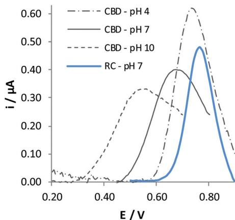
Fig. 3 DPV responses recorded at the bare Gr electrode in 0.1 mM solutions of either CBD or RC, 0.1 M BRB and  $\text{CH}_3\text{CN}$  in 5:2 v/v ratio. The voltammograms reported are subtracted for the relevant signal in the absence of the analyte.
