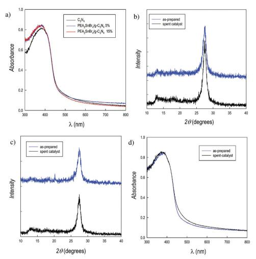
Fig. 2 (a) UV-vis spectra of pristine  $g-C_3N_4$  and  $PEA_2SnBr_4/g-C_3N_4$  composites; (b) XRD pattern of  $PEA_2SnBr_4/g-C_3N_4$  5% composite as-prepared and after the H2 photogeneration experiment (spent catalyst); (c) XRD pattern of PEA2SnBr4/g-C3N4 15% composite as-prepared and after the H2 photogeneration experiment (spent catalyst); (d) UV-vis spectra of  $PEA_2SnBr_4/g-C_3N_4$  5% composite as-prepared and after the  $H_2$  photogeneration experiment (spent catalyst).
