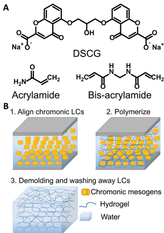
Fig. 1 Schematic of the templating process. (A) Chemical structure of DSCG and monomers. (B) Illustration of the synthesis of anisotropic hydrogels templated by chromonic liquid crystals.
