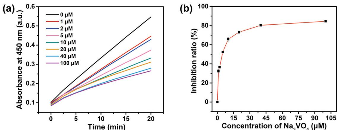
Fig. 4 (a) Kinetics curves of the absorption of ALP responsive reaction systems in the presence of various concentrations of Na<sub>3</sub>VO<sub>4</sub>. (b) The dependence of the inhibition ratio on the concentration of Na<sub>3</sub>VO<sub>4</sub>. Each error bar shows the standard deviation of three independent measurements.
