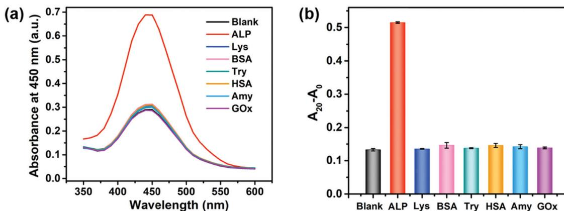
Fig. 3 (a) Typical absorption spectra and (b) the relative change of the absorption of OPDox catalyzed by 2.5 μg mL<sup>-1</sup> of the 2D-MOF with 2 μM of PPI in the absence and presence of 20 U L<sup>-1</sup> of ALP, and 20 nM of Lys, BSA, Try, HSA, Amylase, and GOx. *A*<sub>20</sub> and *A*<sub>0</sub> were the absorption of OPDox at 450 nm at 0 min and 20 min, respectively. Each error bar shows the standard deviation of three independent measurements.
