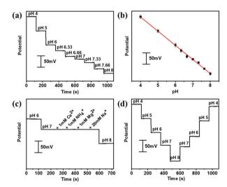
Fig. 2 The electrochemical performance of Au/PANI fiber-based pH sensor in standard McIlvaynes buffers versus Au/Ag/AgCl reference electrode. (a) The open circuit potential performance of fiber-based pH sensor to different pH ranging from 4 to 8. (b) Calibration curves for pH sensor. (c) The selectivity of fiber-based pH sensor. (d) The repeated performance of fiber-based pH sensor in one complete cycle from pH 4 to 8.
