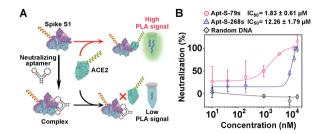
Fig. 5 (A) Schematic illustration of our adapted proximity ligation assay for evaluation of the neutralization efficiency of potential neutralizing aptamers that bind to spike S1. (B) Dose-response neutralization titration curves of spike S1 using two aptamers targeting spike S1 and a random DNA as a negative control. The spike S1-DNA probe was pretreated with different concentrations of neutralizing aptamers for 10 min, and then tested using our adapted proximity ligation assay
