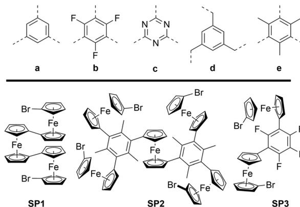
**Scheme 1** (Top) Preparation of tris-phosphanes **1a-d** and complexes **[(1a-c)E]**. (I) Pd precatalyst, THF, r. t.; (II) *n*BuLi, Ph<sub>2</sub>PCL, THF, -80 °C to r. t.; (III) [E]-X ([E]-X = BH<sub>3</sub>·SMe<sub>2</sub> or [AuCl(tht)]), CH<sub>2</sub>Cl<sub>2</sub>, r. t.; (Bottom) crystallographically characterised side products obtained during the syntheses of **4d** (SP1), **4e** (SP2), and **4b** (SP3). For their solid-state structures, see Fig. S3.†
