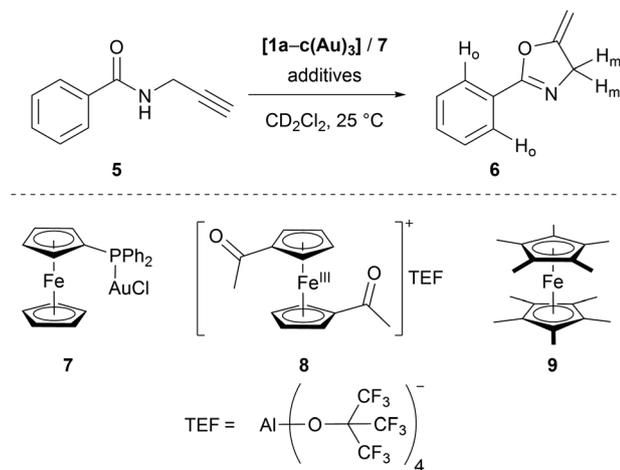
Scheme 2 Gold(I)-catalysed ring-closing isomerisation of *N*-(2-propyn-1-yl)benzamide **5** to oxazoline **6** (top, labelled protons used for following the reaction), including alternative mononuclear (pre-) catalyst **7**, oxidant **8**, and reductant **9**.
