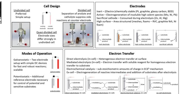
Fig. 1 Modes of operation for electro-organic synthesis and electrochemical facts at a glance. Photography reproduced with permission from ref. 7. Copyright 2018 ACS.
