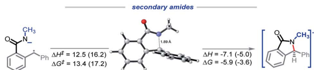
Scheme 18 Computed activation and reaction enthalpies and Gibbs energies for the cyclization of secondary amide 1r . Numbers in parentheses are for primary amide 1a . All numbers reported in \text{kcal mol}^{-1} .
