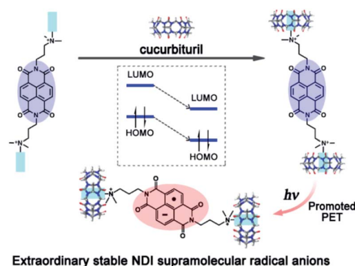
Fig. 13 NDI •− stabilized by the electrostatic effect of cucurbit[7]uril. Reproduced from ref. 63 with permission from Royal Society of Chemistry, Copyright 2015.
