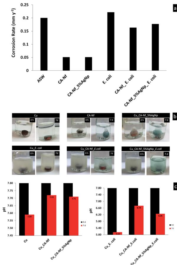
Fig. 7 Cu, Cu coated CA-Nf and Cu coated CA-Nf with 5% AgNps in the ASW and ASW inoculated with *E. coli* for 7 days. Also, Fig. 7 shows photographs of the Cu discs weight loss analysis and (c) pH changes.
