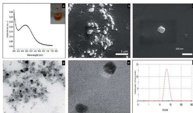
Fig. 1 (a) UV-vis absorption spectrum recorded from aqueous AgNO<sub>3</sub> – the cell free extract of the *Lysinibacillus* sp. NOSC culture medium after 24 h time of reaction, inset shows the color the reaction mixture (b and c) SEM images of the AgNps (d and e) TEM images of the AgNps (f) DLS analysis of the AgNps.
