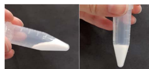
Fig. 1 DES in water emulsion (30 : 70 volume ratio) stabilised by 1.5 wt% OCNF after more than 200 days at room temperature.
