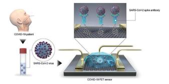
Fig. 4 Schematic diagram of COVID-19 FET sensor operation procedure.<sup>40</sup>
