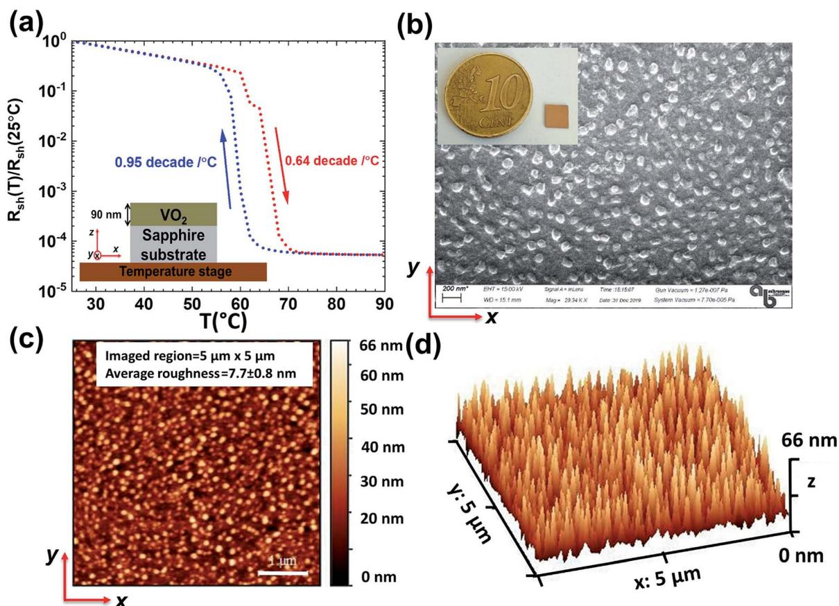
Fig. 1 (a) Electrical characterization of  $\text{VO}_2$  ultrathin film (“sample A”) as a function of temperature during heating (red colored) and cooling (blue colored). The inset depicts the  $x$ – $z$  side view of the “sample A” on a temperature stage. (b) Scanning electron microscope image of the “sample A”. Inset: Optical image of the “sample A” and size comparison with a coin of 10 eurocents. (c) 2D and (d) 3D atomic force microscopy images of the “sample A”.
