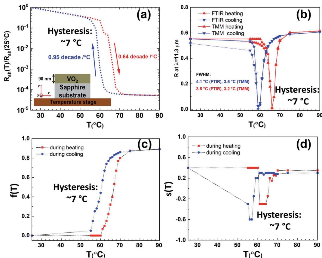
Fig. 3 Hysteretic behaviors observed in (a) normalized electrical resistance, (b) experimental (FTIR) and simulated (TMM) reflectivity ( $R$ ) from the "sample A" at  $\lambda = 11.3 \mu\text{m}$ , effective-medium theory parameters of (c)  $f(T)$  and (d)  $s(T)$  as the applied temperature increases and decreases. Inset (a) is  $x$ - $z$  side view of "sample A" on a temperature stage.
