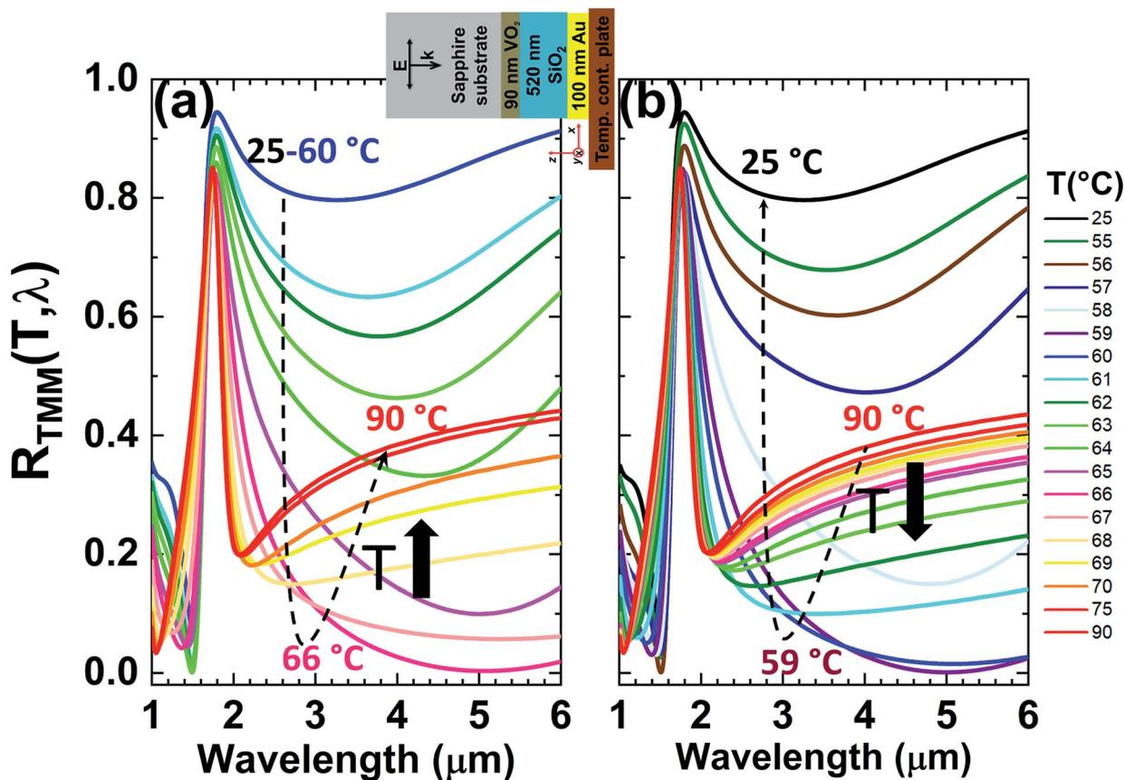
Fig. 6 Simulated spectral reflectivity of  $R_{\text{TMM}}(T, \lambda)$  of the "sample C" during (a) heating and (b) cooling cycles. Inset (a) is  $x$ - $z$  side view of the simulated "sample C" on the temperature  $T_{\text{TMM}}$  and illumination conditions. The dashed black curved lines drawn to guide the eye represent the trajectories of the temperatures during heating and cooling. The colored horizontal lines on the right refer to the temperatures applied during heating and cooling.
