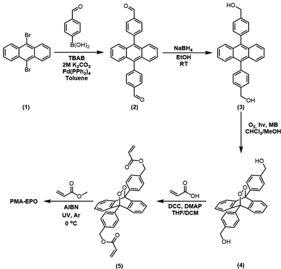
Fig. 1 Synthesis scheme for the monomer 5.
