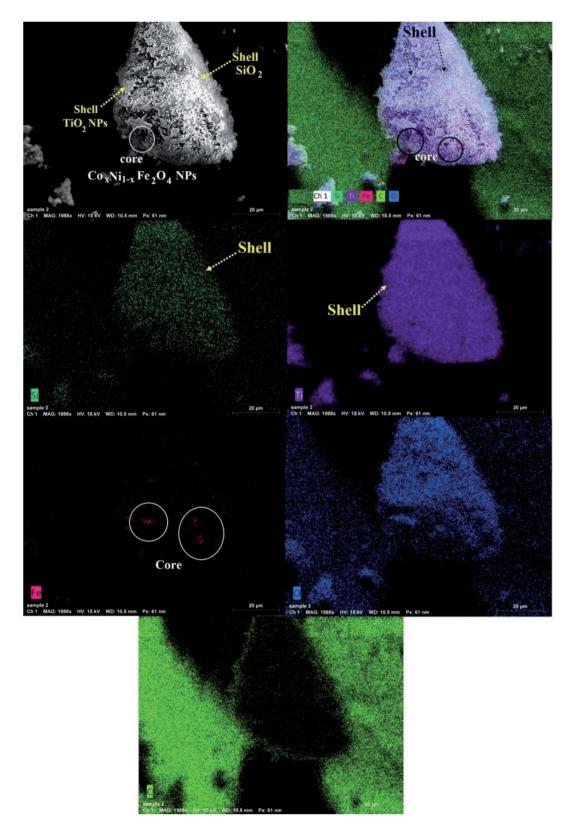
Fig. 3 SEM-EDX elemental mapping of the synthesized  $Co_xNi_{1-x}Fe_2O_4/SiO_2/TiO_2$ ; x=0.9 nanocomposite.
