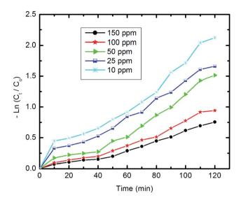
Fig. 11 The first-order kinetics of pyridine degradation (10 mg of composite, 50 ml Py solution, 25  $^{\circ}$ C and pH 7).
