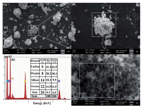
Fig. 2 SEM and corresponding EDX elemental analysis of the synthesized  $Co_xNi_{1-x}Fe_2O_4/SiO_2/TiO_2$ ; x = 0.9 nanocomposite. [A-C] Different magnifications of the core–multi-shell structure. [D] The corresponding EDX elemental analysis of the synthesized nanocomposite.
