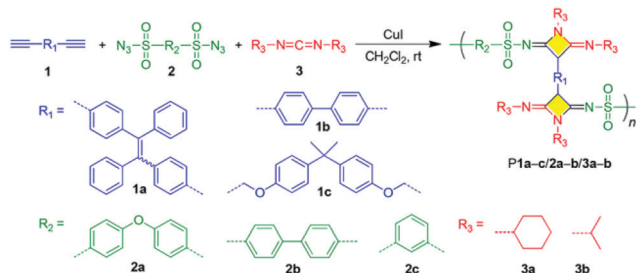
Fig. 11 Three-component polymerization using the small heterocycles route. Adapted from ref. 107 with permission. Copyright (2018) American Chemical Society.
