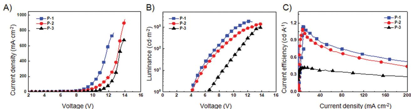
Fig. 6 Electroluminescence performance of different LEDs. (A) Current density–voltage ( $J$ – $V$ ), (B) luminance–voltage ( $L$ – $V$ ) and (C) current efficiency–current density ( $\eta$ – $J$ ) curves.
