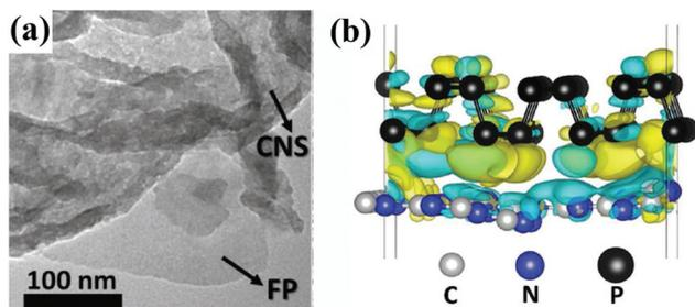
**Fig. 3** (a) TEM image of the as-fabricated P-g-CN heterojunction. (b) Side-view differential charge density map of phosphorene and g-C<sub>3</sub>N<sub>4</sub>. Reproduced from ref. 80 with permission from Wiley-VCH, Copyright 2018.
