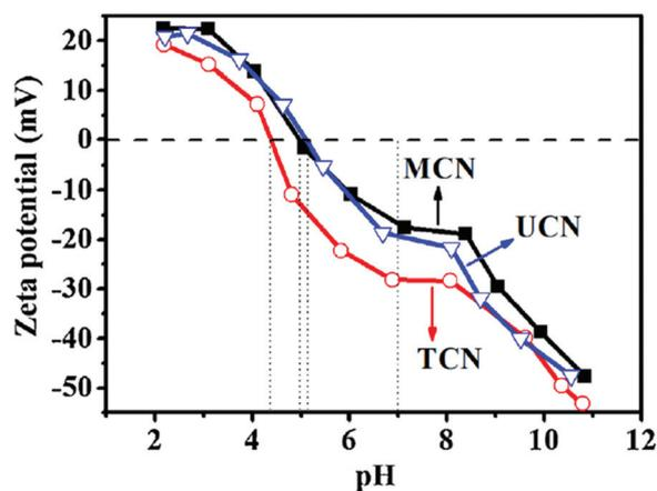
Fig. 7 Measured zeta potential values of  $g\text{-C}_3\text{N}_4$  suspensions prepared from urea (UCN), melamine (MCN) and thiourea (TCN) with varied pH values. Reproduced from ref. 113 with permission from Elsevier, Copyright 2015.
