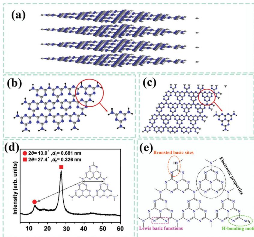
Fig. 6 (a) Illustrations of the two-dimensional layer structure of  $g\text{-C}_3\text{N}_4$ , (b) s-triazine, and (c) tri-s-triazine as the main building blocks of  $g\text{-C}_3\text{N}_4$ . Reproduced from ref. 21 with permission from Elsevier, Copyright 2017. (d) XRD pattern of  $g\text{-C}_3\text{N}_4$ . Reproduced from ref. 24 with permission from Nature Publishing Group, Copyright 2009. (e) Multiple surface physicochemical properties of  $g\text{-C}_3\text{N}_4$ .<sup>25</sup>
