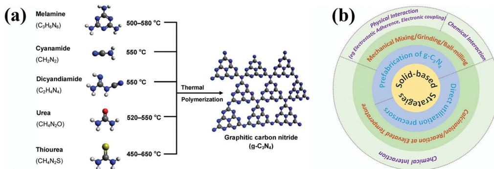
**Fig. 2** (a) Graphical illustration of the general preparation conditions for g-C<sub>3</sub>N<sub>4</sub> from various organic precursors, where the blue, grey, white, red and yellow balls represent N, C, H, O, S atoms, respectively. Reproduced from ref. 41 with permission from the American Chemical Society, Copyright 2016. (b) Synthetic strategies for g-C<sub>3</sub>N<sub>4</sub> composite photocatalysts with interface contacts based on solid-state conditions.
