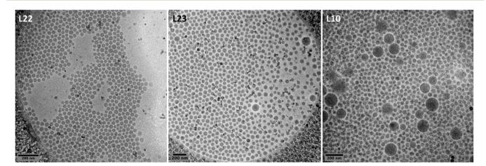
Fig. 5 Cryo-TEM images photos of the latexes obtained during the kinetic study performed at 50 bar with 10 wt% of macroCTA: t = 10 min (L22), t = 20 min (L23) and t = 240 min (L10).
