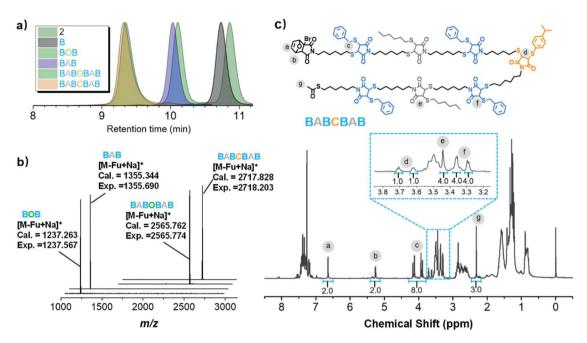
Fig. 4 (a) SEC traces of discrete precursors with palindromic sequences. THF was used as an eluent. (b) MALDI-TOF mass spectra of BOB, BAB, BABOBAB and BABCBAB. (c) The <sup>1</sup>H NMR spectrum of BABCBAB recorded in CDCl<sub>3</sub> (Bruker, 300 MHz, TMS).
