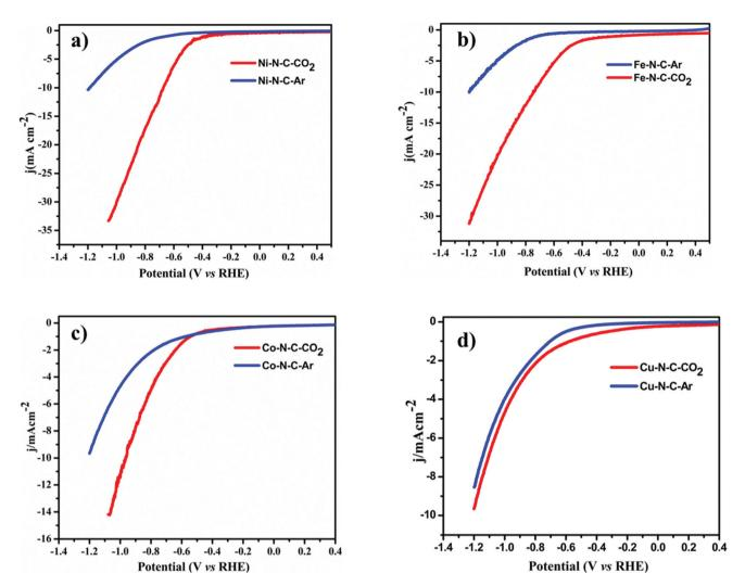
Fig. 4 CO<sub>2</sub> reduction reaction activities. Linear sweep voltammetry of (a) Ni-N-C, (b) Fe-N-C, (c) Co-N-C and (d) Cu-N-C in CO<sub>2</sub>-saturated 0.1 M KHCO<sub>3</sub> (red lines) and in N<sub>2</sub>-saturated 0.1 M KHCO<sub>3</sub> (blue lines) at 5 mV s<sup>-1</sup> in the cathodic direction.
