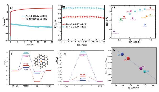
Fig. 6 Long-term stability test (a) and the partial current density (b) for Ni-N-C and Fe-N-C at -0.8 and -0.5 V vs. RHE, respectively. (c) TOF of Ni-N-C and Fe-N-C catalysts compared with other CO<sub>2</sub> to CO reduction catalysts. (d) Calculated free energy diagram for CO<sub>2</sub>RR (d) and HER (e) on the 4-coordinated metal center of nitrogen-doped graphene and (f) the onset potential correlation with the free energy of COOH\*.
