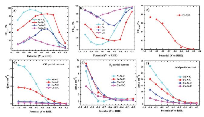
Fig. 5 Electrocatalytic CO<sub>2</sub>RR performance of M-N-C in the H-cell. (a-c) FEs of CO, H<sub>2</sub> and CH<sub>4</sub> and (d-f) the corresponding steady-state current densities of M-N-C in CO<sub>2</sub>-saturated 0.1 M KHCO<sub>3</sub>.
