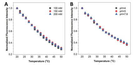
Fig. 4 Functional independence of the HPS/Butter/DSPE-PEG-Biotin nanorod to (A) the influence of salt concentration and (B) the influence of pH, examined using a fluorescence spectroscopy. Sample solutions were excited at 375 nm. Fluorescence intensity under different conditions was normalized to that at 20 °C. NaCl was used as the salt. Citric acid and Na<sub>2</sub>HPO<sub>4</sub> were used to prepare the buffer solution with different pH.
