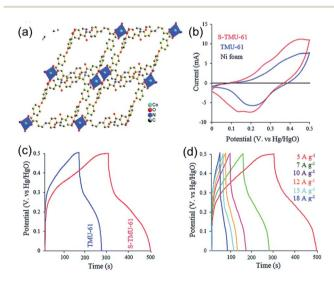
Fig. 14 (a) Topological diagram of TMU-61. (b) CV curves of TMU-61, S-TMU-61, and Ni foam at a scan rate of 25 mV s<sup>-1</sup>, (c) GCD curves of TMU-61 and S-TMU-61 electrode materials at a current density of 5 A g<sup>-1</sup> and (d) GCD curves of S-TMU-61 at different current densities. Reproduced with permission. 118 Copyright © 2019 The Royal Society of Chemistry.
