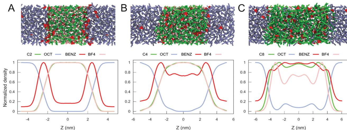
**Fig. 4** Extraction of benzene from petroleum oil: snapshots of the final state of the petroleum oil/IL biphasic system and normalized density profiles for C2 (A), C4 (B) and C8 (C). Colour code: In green, the cation, composed of the imidazolium ring and the alkyl tail. In pink, the beads correspond to the anion. In violet, the octane molecules and in red, the molecules of benzene.
