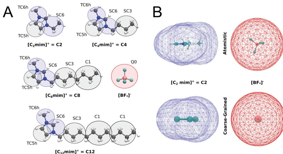
**Fig. 1** Coarse-grain representations of imidazolium based ILs. (A) The Martini bead types and sizes of each bead are indicated. T and S prefixes mark the beads that use tiny and small beads. Blue and red colors indicate positively and negatively charged groups, respectively, while the gray color indicates the apolar groups. (B) Molecular surfaces (also called Connolly surfaces) of atomistic and coarse-grained structures of the C2 cation and the  $[\text{BF}_4]^-$  anion.
