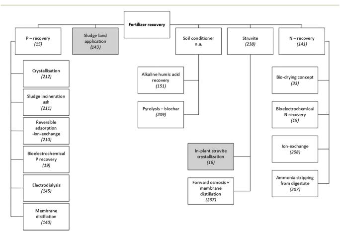
Fig. 3 Examples of technologies to recover fertiliser from municipal WWTPs. Since a detailed presentation and discussion of these technologies is beyond the scope of this paper, scientific publications that explain or review them are referenced. Grey shading indicates techniques that have applied on a large scale municipal WWTPs. Unshaded boxes show technologies that are not widely applied. 15,16,19,33,140,141,143,145,151,207-212,237,238
