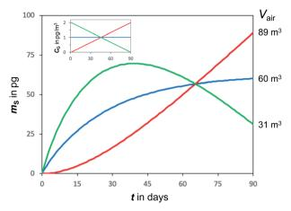
Fig. 9 Simulated uptake curve for a compound with log  $K_{PUF-G}$  of 5.5 in a PUF-PAS during 90 days of constant (blue), increasing (red) and decreasing (green) air concentrations.
