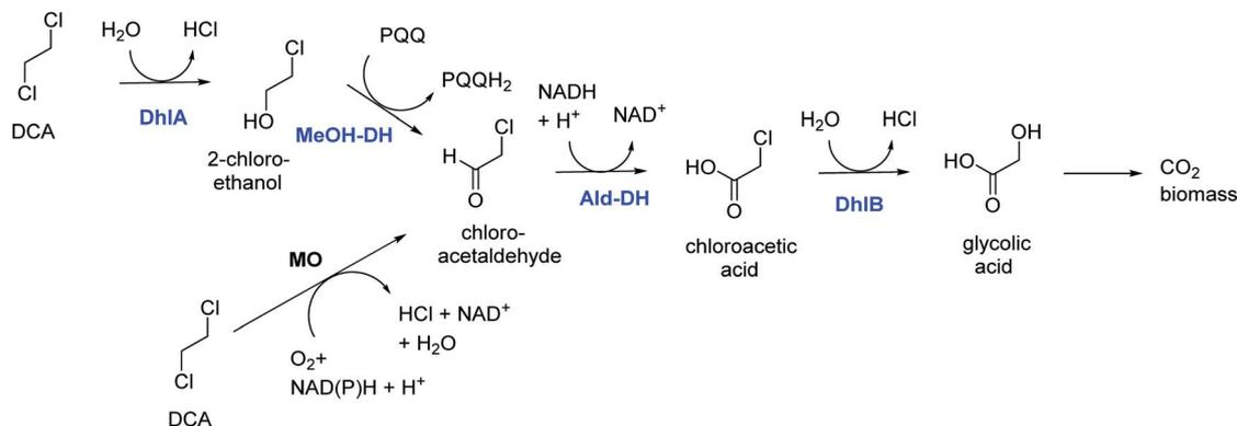
Fig. 1 Aerobic catabolic pathways for 1,2-dichloroethane.<sup>6,27</sup> Enzymes of the *Xanthobacter autotrophicus* pathway are indicated in blue: DhlA, haloalkane dehalogenase; MeOH-DH, methanol dehydrogenase; Ald-DH, chloroacetaldehyde dehydrogenase; DhlB, haloacid dehalogenase. Monooxygenase (MO) – mediated conversion leads to chloroacetaldehyde.
