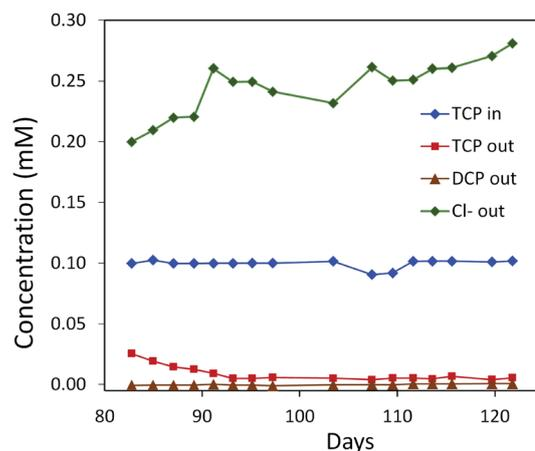
Fig. 6 Degradation of TCP by a mixed culture of *P. putida* strains MC4-5221, MC4-5221, MC4-1331 and *A. radiobacter* AD1 in a laboratory-scale aerated packed bed bioreactor operated in a continuous mode. Packing material was sintered glass and data were collected after an initial 80 day acclimation period. TCP loading rate 0.40–0.44 mg h<sup>-1</sup> l<sup>-1</sup>; residence time 23 h; removal increasing to 95%.<sup>40,62</sup>
