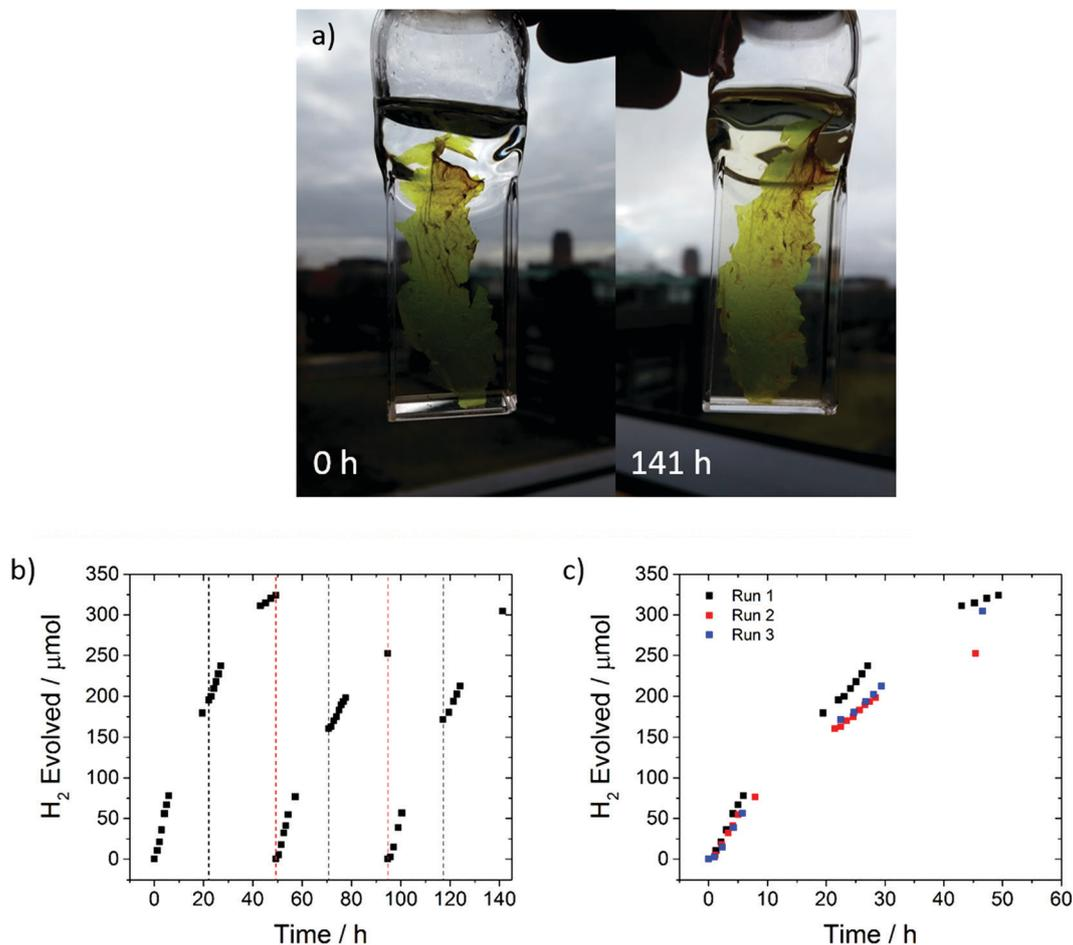
Fig. 6 (a) Images of free-standing film suspended in 5 vol% TEA before and after photocatalytic experiment; (b) hydrogen evolution of free-standing film of **FS-TEG** from a 5 vol% TEA mixture under  $\lambda > 420$  nm irradiation over a period of 141 hours with intermittent degassing (black dashed lines) and replacement of scavenger mixture (red dashed lines) (300 W Xe light source); (c) direct comparison of hydrogen evolution runs after replacing the scavenger mixture.
