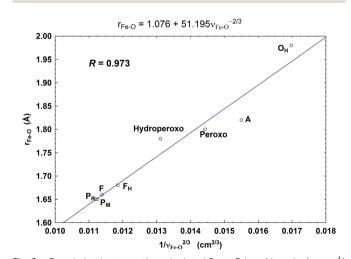
**Fig. 9** Correlation between the calculated Fe<sub>a3</sub>–O bond lengths ( $r_{\rm Fe-O}$ , Å) and the corresponding Fe<sub>a3</sub>–O stretch frequencies ( $1/\nu_{\rm Fe-O}^{2/3}$ , based on Badger's rule) for the eight DNC state structures studied.<sup>59</sup> Reprint with permission from Fig. 7 of ref. 59, copyright© 2019 American Chemical Society.
