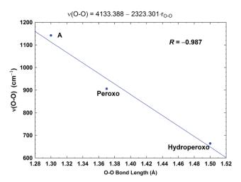
Fig. 10 Correlation between the calculated O–O stretching frequencies  $(\nu(O-O), \, cm^{-1})$  and the O–O bond lengths  $(r_{O-O}, \, \dot{A})$ . Taken with permission from Fig. 6 of ref. 59, copyright © 2019 American Chemical Society.
