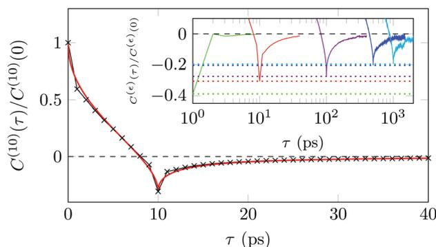
**Fig. 14** Measured displacement-autocorrelation function (black crosses) compared with the theoretical FBM prediction for  $\alpha = 0.47$  and  $\varepsilon = 10$  ps (red line). The inset shows the dependence of the measured displacement autocorrelation function on the binning size  $\varepsilon$  for values of  $\varepsilon$  of 1 ps (green), 10 ps (red), 100 ps (violet), 500 ps (blue) and 1000 ps (light blue).
