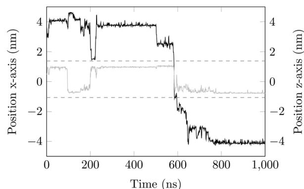
Fig. 6 DOX displacement along the  $x$ -axis for one trajectory (black) and along the channel height (grey), with COM positions shown every ns.
