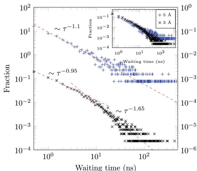
**Fig. 13** Normalised frequency of escape events from the circle of radius  $r_{\text{esc}}$  in the  $(x,y)$ -plane for  $r_{\text{esc}} = 3$  Å (black, left axis) and  $r_{\text{esc}} = 5$  Å (blue, right axis), with  $\tau_{\text{esc}} = 0.5$  ns for both panels. Both distributions are shown together in the inset (sharing the same y-axis).
