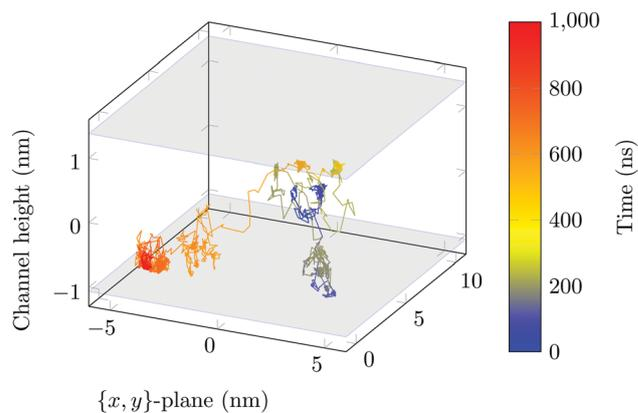
**Fig. 3** Sample 3D trajectory. Position of the COM of the DOX molecule is shown every 200 ps. The grey surface planes indicate the average position of the COM of the hydrogen surface atoms. The colour of the trajectory shows the time evolution (shown in ns).
