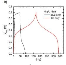
Fig. 5 Simulated electrode response under galvanostatic charge—discharge at 1689  $\mu$ A (2 A g<sup>-1</sup>) for 1\_2 electrodes. (a) At steady operation (after long cycling), and (b) for idealized cases where LS is confined in electrode domain in only solid (sLS) or dissolved (LS) form.
