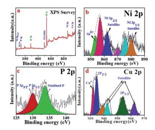
Fig. 4 (a) XPS survey spectra of Cuf@Ni<sub>5</sub>P<sub>4</sub>, and high-resolution deconvoluted XPS sspectra for: (b) Ni 2p; (c) P 2p; and (d) Cu 2p.
