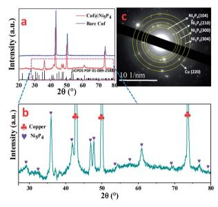
Fig. 2 (a) XRD pattern for Cuf (blue) and Cuf@Ni<sub>5</sub>P<sub>4</sub> (red); (b) scaled image of XRD of Cuf@Ni<sub>5</sub>P<sub>4</sub>; and (c) SAED pattern for Cuf@Ni<sub>5</sub>P<sub>4</sub>.
