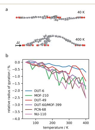
Fig. 5 Structural snapshots of the ligand subunit in NU-110 at 40 and 400 K, where C gray; O red; H white (a). Relative radius of gyration of the oxygen atoms of the largest ligand subunits over the temperature range 40–400 K (b).
