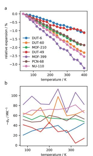
Fig. 2 Relative expansion of the investigated MOFs (a). Volumetric thermal expansion coefficient,  $\alpha_V$ , calculated over the temperature range, computed for intervals of 40 K (b).
