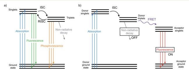
Fig. 1 (a) Representative photophysical pathways of an organochalcogen chromophore/fluorophore include absorption, fluorescence, intersystem crossing (ISC), reverse ISC, phosphorescence, and non-radiative decay. (b) Representative photophysical pathways of an organochalcogen fluorescent probe that is off when non-radiative decay occurs through triplet quenching, and on when Förster Resonance Energy Transfer (FRET) occurs to a fluorescent acceptor.
