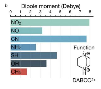
Fig. 4 (a) Total and projected density of states of ODABCO $-NH_4Br_3$ , MDABCO $-NH_4Br_3$  and MDABCO $-NH_4I_3$  obtained with PBESol0-D3. The red line (dash) is the Fermi energy, which is set at the top of the valence band of each material. (b) Variance of dipole moment for DABCO cations substituted with a number of organic groups (functions).
