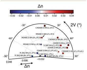
Fig. 2 Computed birefringence  $\Delta n$  and 2V angle of metal-free perovskites at their experimental volume and lattice constants.  $\Delta n$  is plotted on the radial axis and using the colour-bar, with red indicating positive  $\Delta n$ . Values of n are given in Table S3 of the ESI.† The 2V angles provide information about the nature of the birefringence in biaxial crystals.
