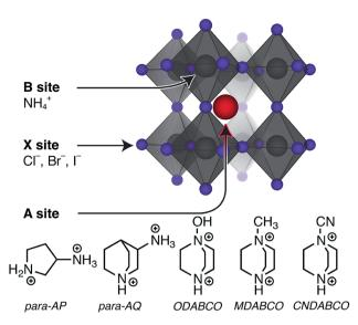
Fig. 1 Polyhedra representation of a metal-free ABX<sub>3</sub>-type perovskite, where A can be one of the four organic cations (also shown by the red ball), B is  $NH_4^+$  (grey ball) and X the halide ion, *i.e.*  $Cl^-$ ,  $Br^-$  and  $I^-$  (purple balls). The nature of the A cation is also shown.
