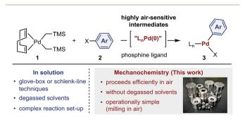
Scheme 1 Synthesis of palladium-based oxidative addition complexes involving air-sensitive palladium(0) intermediates.
